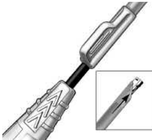
Figure 5. Sheath's tab aligned with the arrows on the probe handle.
